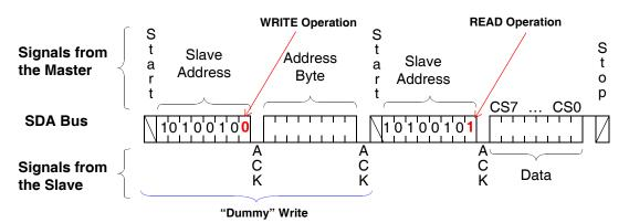
Figure 19. CONSTAT Register Read Command Sequence
