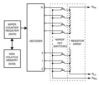
Figure 6. DCP Internal Structure
