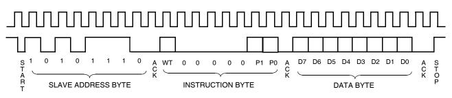
Figure 9. DCP Write Command Sequence
