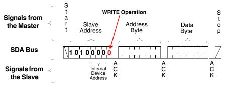
Figure 12. EEPROM Byte Write Sequence
