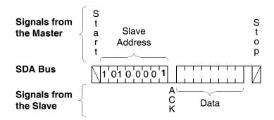
Figure 14. Current EEPROM Address Read Sequence
